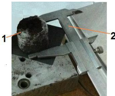
Fig. 2 – The measurement of the plug parameters: 1 – plug; 2 – caliper.
